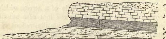
FIG. 2.—Section at Niagara Falls, showing the strata cut through by the action of the Fall. Thickness of beds about 250 feet.
